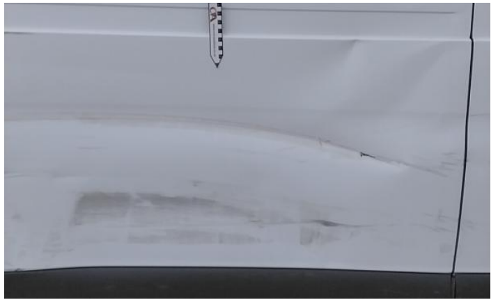
28: Qtr Panel osr Dented With Paint Damage
