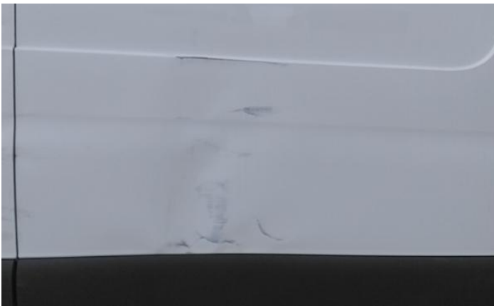
29: Qtr Panel osr Scratched Over 25mm Thru Paint
