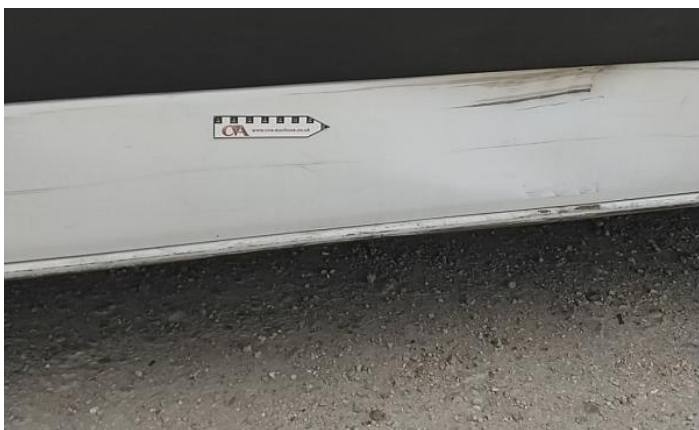
9: Door nsf Dented Over 30mm
