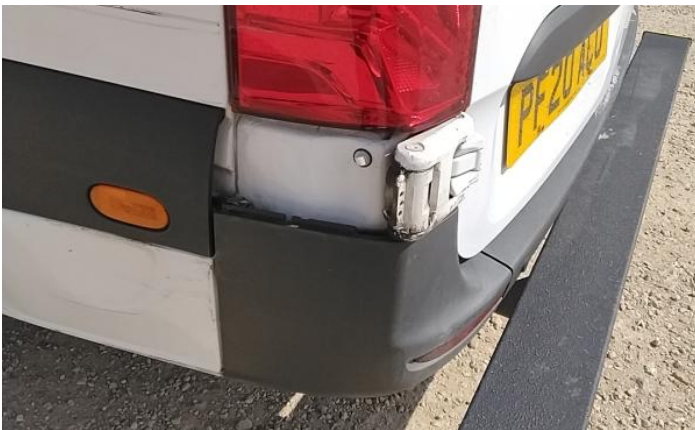
17: Sill ns Dented With Paint Damage
