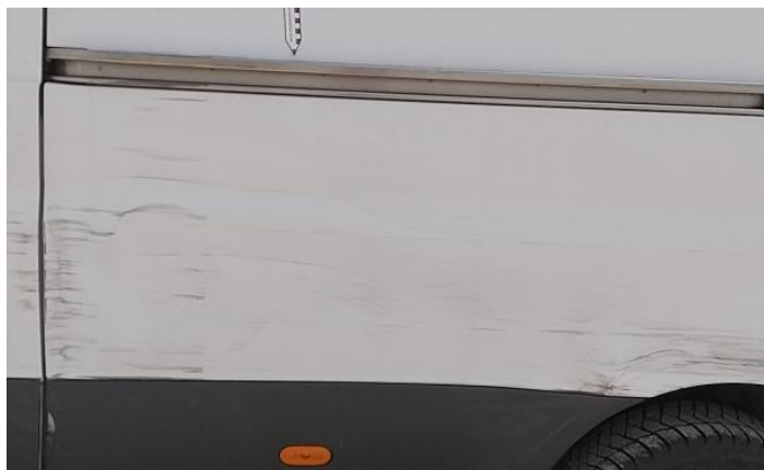
12: Door nsr Dented Over 30mm
