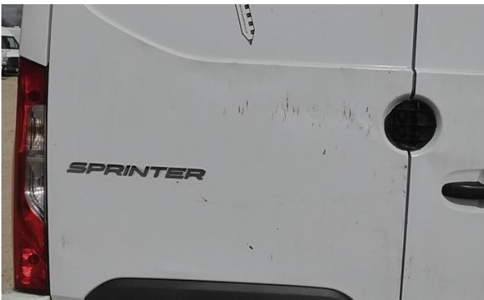
21: Door nsr Dented Over 30mm
