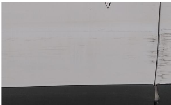
10: B Post ns Dented With Paint Damage
