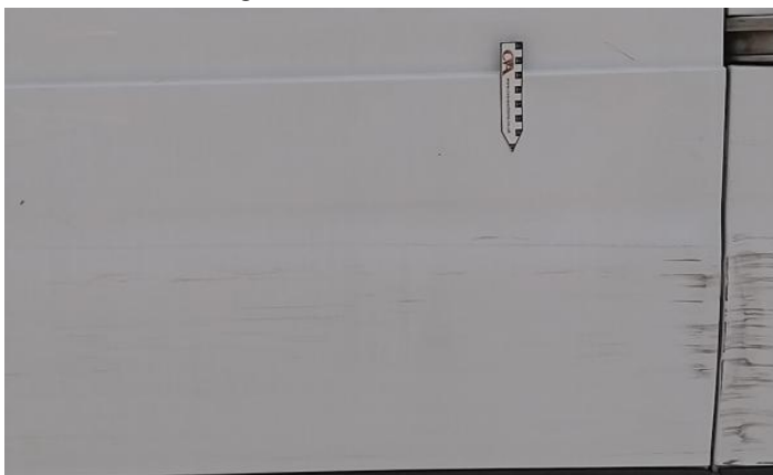
11: Door nsr Dented With Paint Damage
