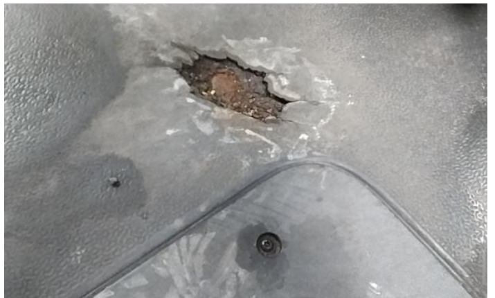
30: Qtr Panel osr Dented With Paint Damage
